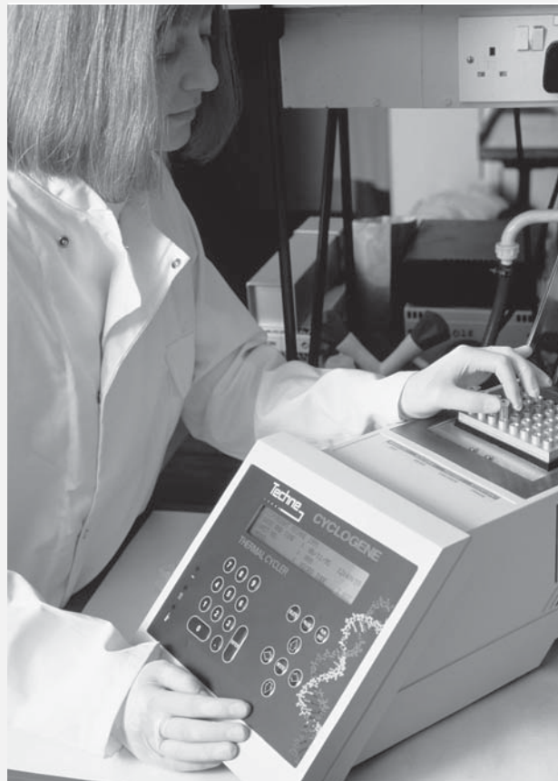
Figure 3.1 A lab technician performs a PCR, which is used to make multiple copies of DNA. Blood donations are tested for WNV using a form of PCR.
